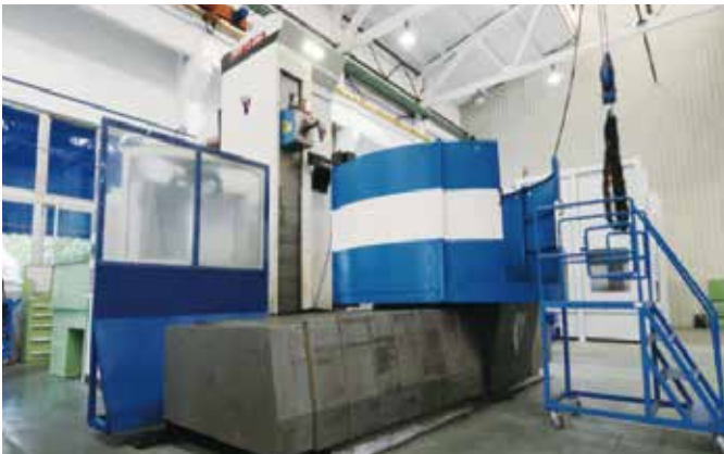
➤ WFT13 boring and milling horizontal machining center with five-axle four-linkage control
