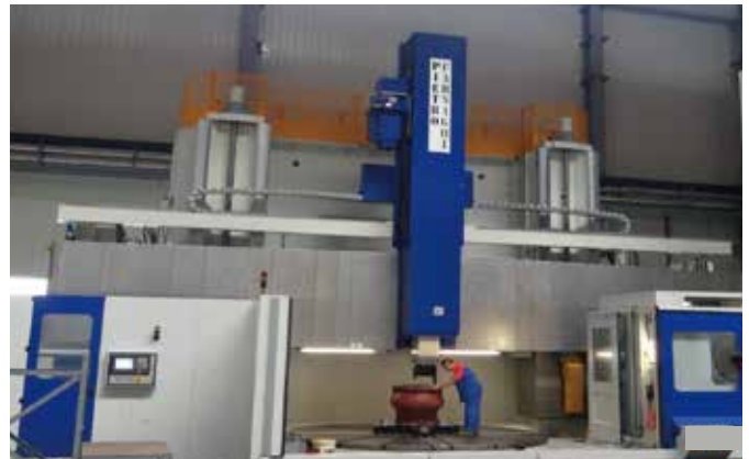
➤ AC46TM-4000 heavy-duty high precision vertical lathe-milling machining center
