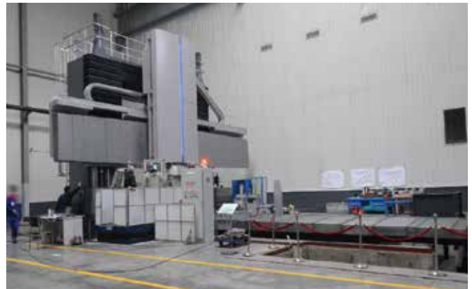
➤ ProfiMill 4000/100-T Gantry boring and milling machining center with six-axle five-linkage control
