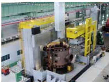
➤ Floor Boring and Milling machining center with nine-axle five-linkage control
